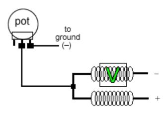
Depending on what the right lug of the pot is connected to, hot or negative ground will determine which coil is affected by the signal at the intersection. Please note again that when connected to hot, it must run to the switchable hot (the guitars pickup selector switch) so there is NO hot signal going to this pickup when it is not selected.
