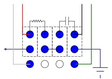
*LEAD: BOTH COILS FULL + RC* RED – OUTPUT BLACK – GROUND
