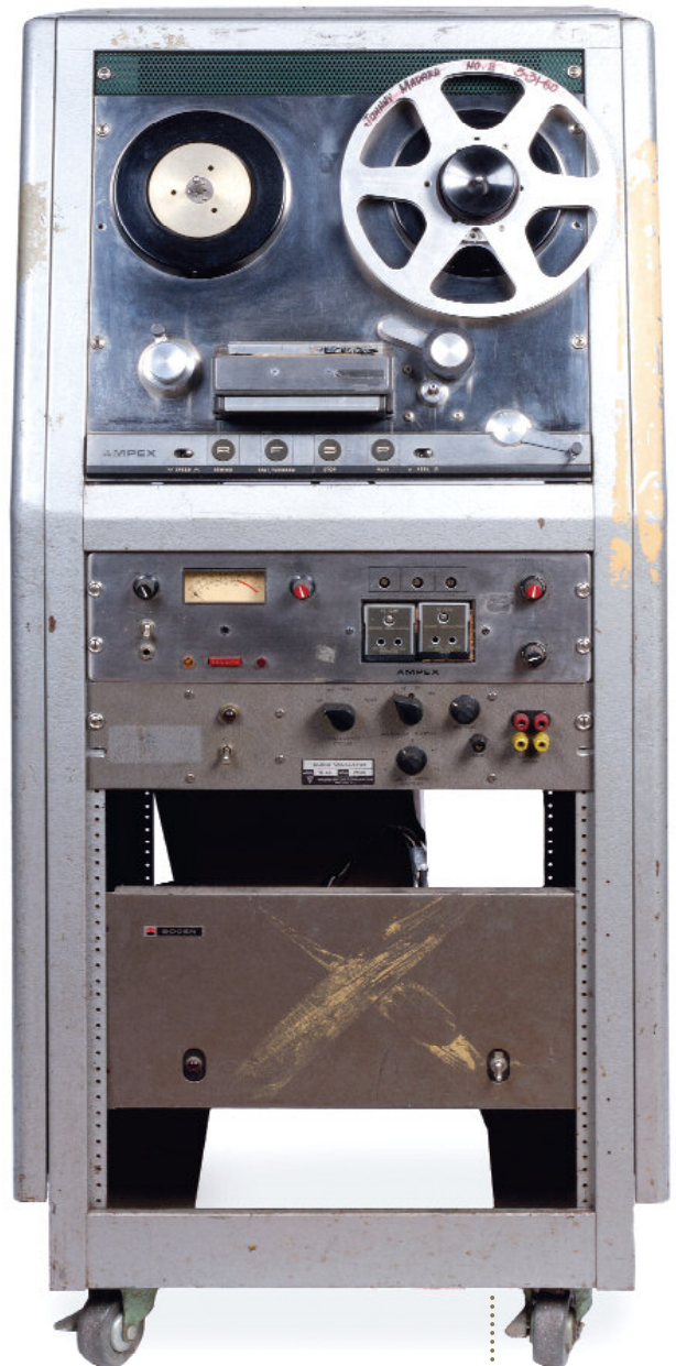
430 LES PAUL RACK A rack on casters containing: an Ampex quarter inch reel, audio electronics model, a pre-stereo mono model; a pitch meter; a Log Corp W66 audio oscillator; and a Bogen tube power amplifier. The back of the unit features two VU meters mounted into a cardboard box, a quick hand-made solution created by Paul. 54 by 25 by 25 1/2 inches
