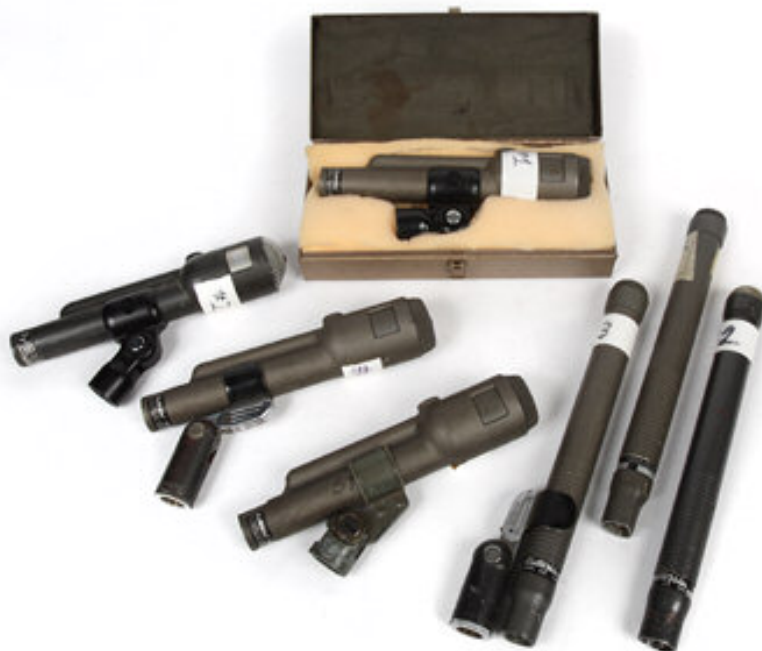
207 LES PAUL MICROPHONES A group of seven Electro Voice microphones, three omnidirectional model 655C and four cardioid model 666 with one cable
