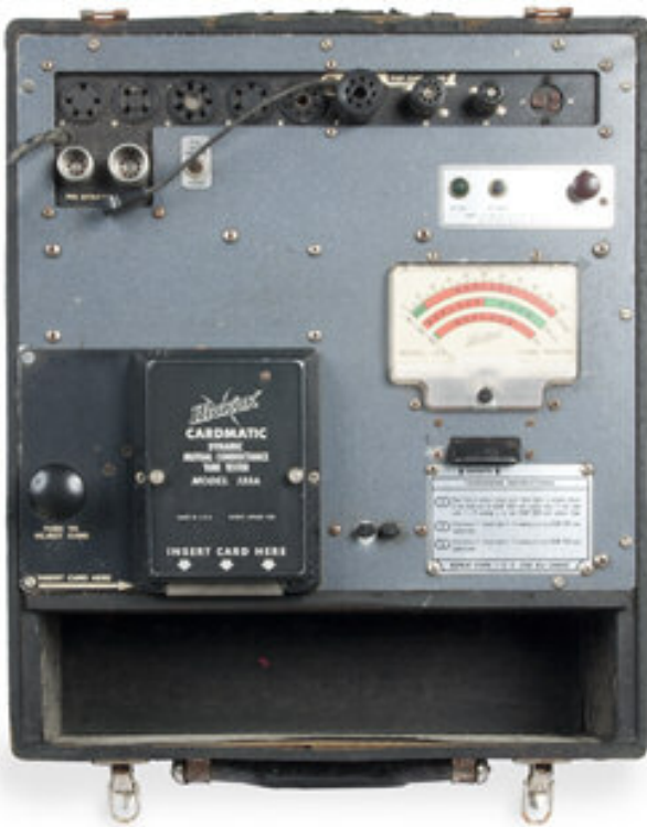
36 LES PAUL TUBE TESTER A Hickok Cardmatic Tube Tester, model 123-A, built into a road case. 9 by 16 1/2 by 20 inches
