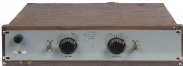
223 LES PAUL ELECTRONICS A Cinema Engineering Co. Program EQ, type 4031-B, with Paul's labels on the back. 5 by 20 by 13 inches
