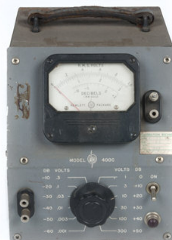
46 LES PAUL TEST METER A Hewlett Packard 400-C decibel test meter, serial number 12152. 6 1/2 by 7 1/2 by 10 inches
