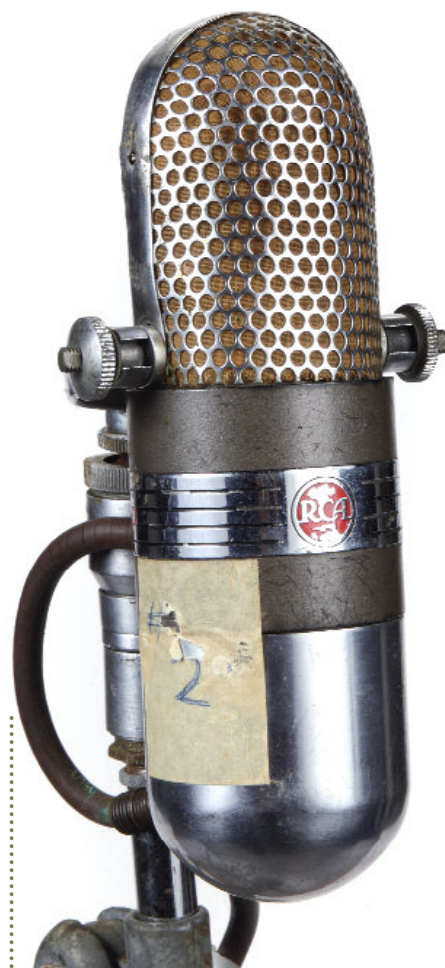
703 LES PAUL MICROPHONE A 1950s RCA model 77D ribbon microphone with a cable.
