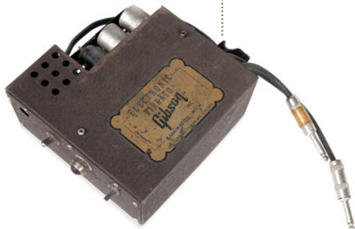
188 LES PAUL EFFECTS A Gibson Electronic Vibrato unit. 3 1/2 by 6 by 6 1/2 inches
