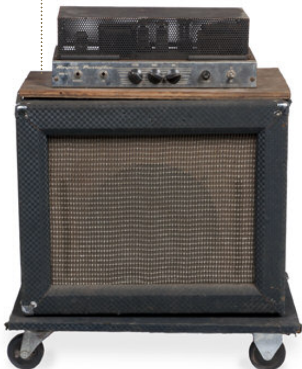
372 LES PAUL BASS AMPLIFIER An Ampeg Portaflex model SB-12 flip top bass amplifier with 12 inch speaker, modified to mount the head externally on a wooden plank with the entire cabinet mounted to a dolly. 30 by 22 1/2 by 14 inches $100-150
